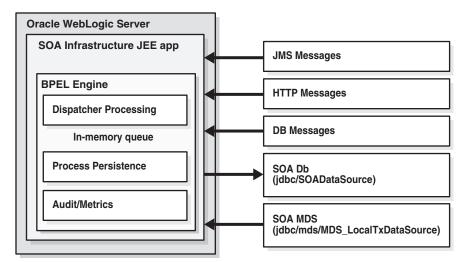
Figure 5–8 Oracle BPEL PM Single-Instance Architecture
