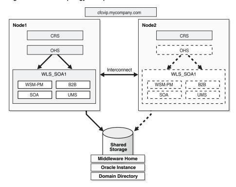
Figure 13–1 CRS Topology Example 1
