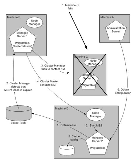
Figure 3–2 Automatic Migration of a Failed Server
