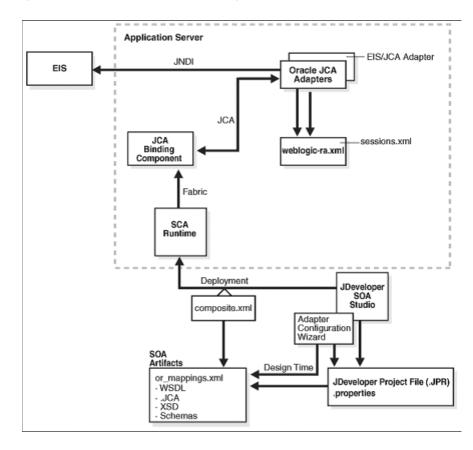
Figure 5–30 Oracle JCA Adapters Single-Instance Architecture
