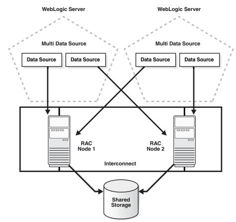
Figure 4-1 Multi Data Source Configuration
