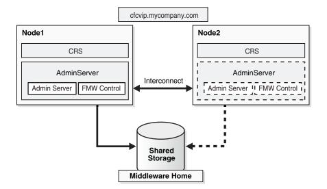
Figure 2–4 Example Active-Passive Cold Failover Cluster Deployment
