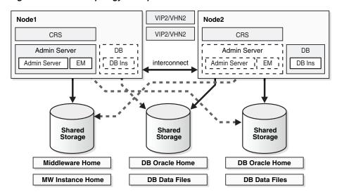
Figure 13–2 CRS Topology Example 2
