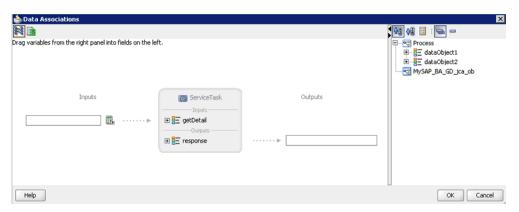
7. Drag and drop dataobject1 (request) to the Inputs field and dataobject2 (response) to the Outputs field, as shown in Figure 1–118.
