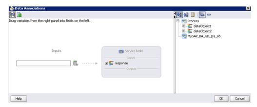
**15.** Drag and drop **dataobject2** (response) to the Inputs field, as shown in Figure 1–125.
