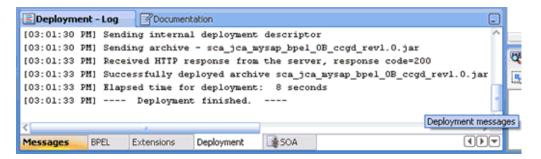
17. After the deployment is successful, open the Oracle Enterprise Manager console and execute the deployed process either in Tree View or XML View to receive a successful response, as shown in Figure 1–88 and Figure 1–89.
