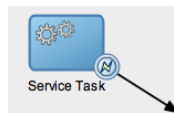
Figure 6–42 The Error Catch Event as a Boundary Event on a Service Task
