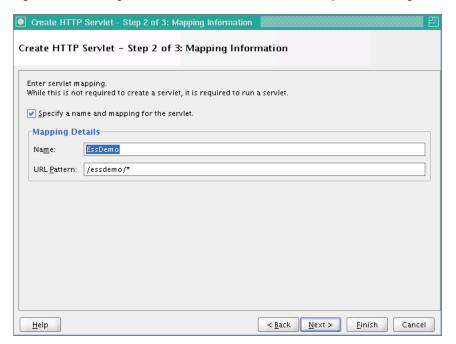
Figure 5-11 Using the Create HTTP Servlet Wizard: Step 2 of 3 Dialog
