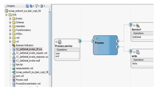
7. Expand the migrated project in the left pane (for example, mysap\_esdsun9\_jca\_ bpm\_ccgd\_OB) and then double-click the **composite.xml** file to verify that the project opens without any errors.
