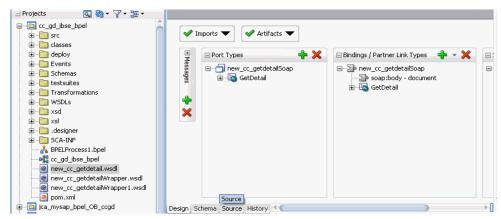
Change the <soap:address location> element to point to the system and port number where 12c is running.
