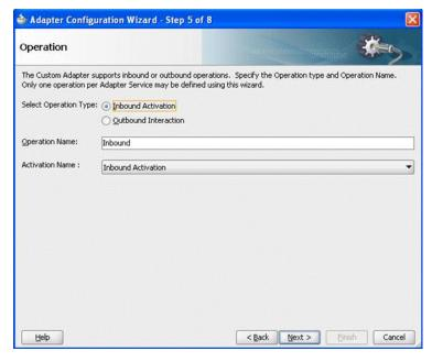
If the user selects Outbound Interaction on the Custom Adapter's Operation page, a list of Interaction Class names (or translated display names as seen in this example) is displayed from the customAdapter-config.xml, from which the user can choose.
