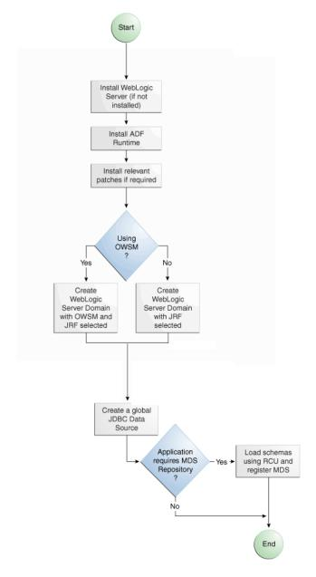
Figure 4–1 Preparing the Application Server Flow Diagram
