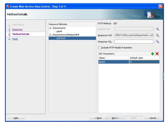
Figure 5–2 Method Details Page of the Create Web Service Data Control Wizard
