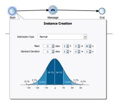
Figure 8-1 Simulation - Normal Distribution in a Start Event
