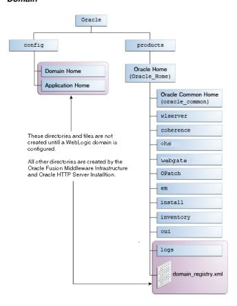
Figure A-1 Sample Oracle HTTP Server Directory Structure in a WebLogic Server Domain
