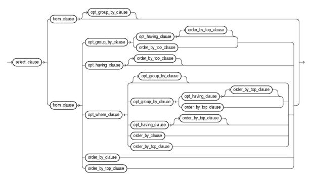
The sfw\_block is made up of the following parts:
