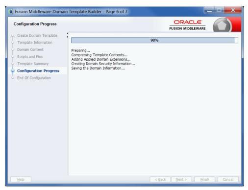
The Configuration Progress screen displays status messages during the template creation process. The Domain Template Builder generates a JAR file that contains all the components required to generate a new WebLogic domain, including the template settings that you provided.
