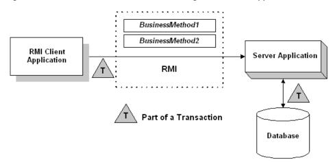
Figure 2–2 How Transactions Work in a WebLogic Server RMI Application
