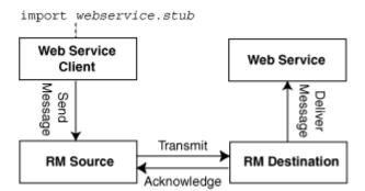
Figure 8–1 Web Service Reliable Message Exchange
