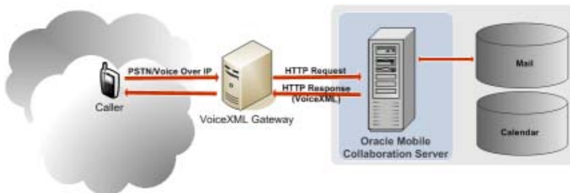
Figure 2–9 The Network Flow for Oracle Voice Access
