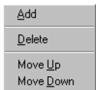
The Add option causes the field to be added to the search criteria table at the bottom of the Search Builder window.
