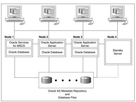
Figure 3–2 Active/Passive (Standby) Four-Node Configuration
