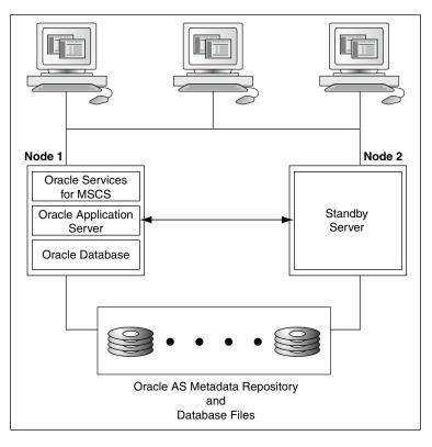
Figure 3–1 Active/Passive (Standby) Two-Node Configuration
