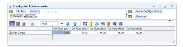
On the Breakpoint Administration view, for a Configuration/Cluster intersection, set the Index to Average to be used by the Breakpoints algorithm for sorting data points into grades. The number of configurations available in this view is based on the Maximum Number of Clusters configured in the Grade Plug-In. Only one configuration is required for use with the breakpoints method.
