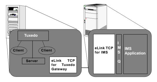
The configuration definition of the eLink TCP for Tuxedo gateway in the remote BEA Tuxedo system maps BEA Tuxedo local services to remote services provided by the IMS gateway. Each remote service corresponds to an IMS server transaction. Service requests issued by clients in the BEA Tuxedo system are routed through the eLink TCP for Tuxedo gateway to the eLink TCP for IMS gateway for processing by the appropriate IMS server transaction.
