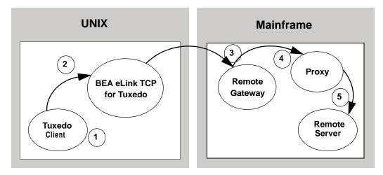
Figure 4-1 Security Checking for Tuxedo to Mainframe Transactions
