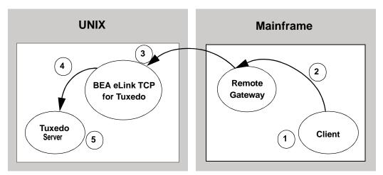
Figure 4-2 Security Checking for Mainframe to Tuxedo Transactions
