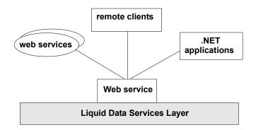
To expose data services through a web service interface, add the Liquid Data control to a web service project in WebLogic Workshop. Then add data service functions from the control to your web service. The web service function needs only to pass through the results of the data service function, as shown in the following sample of generated code:
