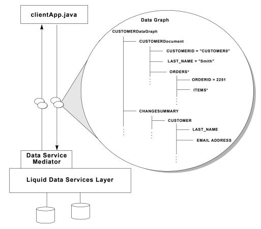
Figure 2-1 SDO Components with Data Graph
