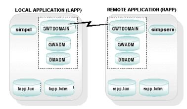
Figure 2-4 Local and Remote Applications in simpapp
