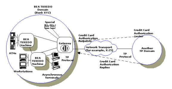
Figure 1-3 High-level View of Two Communicating Domains
