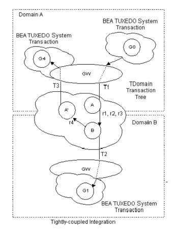
Figure 3-6 Transaction Tree for TDOMAIN Environment
