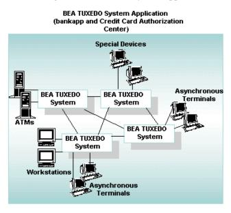
Figure 2-2 Combining Two BEA Tuxedo System Applications
