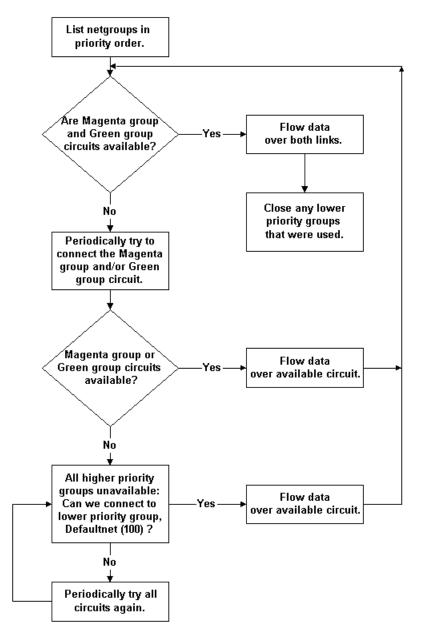
Figure 8-1 Flow of Data over the BRIDGE
