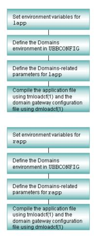
The following diagram shows which sections of the UBBCONFIG and DMCONFIG files you need to configure for a 2-domain application. One domain represents the local domain; the other, the remote domain.
