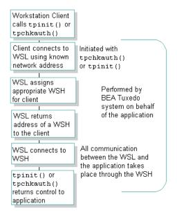
The client connects to the WSL process using a known network address. The process for establishing this connection is initiated when the client calls tpchkauth() or tpinit(). The WSL returns the address of a WSH to the client, and then notifies the Workstation Handler process of the connection request. The WSC connects to the WSH. All further communication between the WSC and the application takes place through the WSH.
