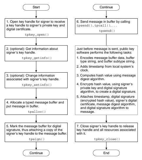
Figure 3-3 Procedure for Sending Signed Messages
