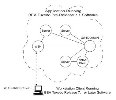
Figure 2-5 Older WSH Operating with Workstation Client
