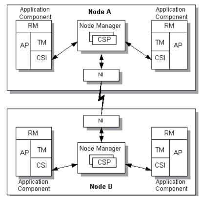
Figure 1-2 Basic BEA TOP END System Architecture
