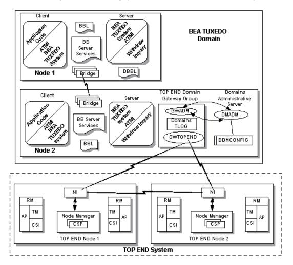
Figure 1-3 Connecting Systems with the TOP END Domain Gateway
