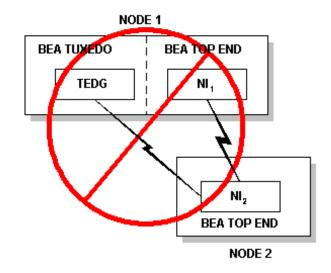
Figure 4-3 Invalid Multi-node TEDG Configuration
