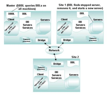
Both servers have a role in managing faults. The DBBL coordinates the state of other active machines in the application. Each BBL communicates state changes in the MIB, and sometimes sends a message to the DBBL indicating all is OK on its host machine.
