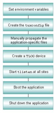
Figure 1-1 Startup and Shutdown Tasks
