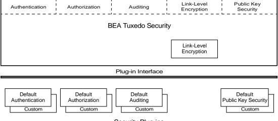
Figure 1-1 BEA Tuxedo ATMI Plug-in Security Architecture
