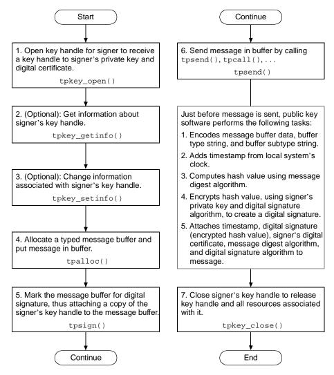
Figure 3-3 Procedure for Sending Signed Messages
