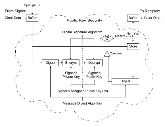
Figure 1-7 ATMI PKCS-7 End-to-End Digital Signing
