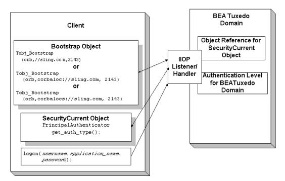
Figure 3-2 How Password Authentication Works
