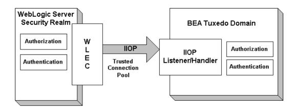
Figure 1-2 Single Sign-on in the CORBA Security Environment
