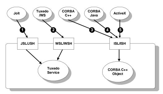
Figure 1-2 Remote Client and Server Interoperability
