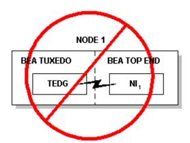
Figure 4-4 Invalid Single-node Configuration
