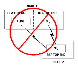
Figure 4-3 Invalid Multi-node TEDG Configuration
