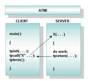
Figure 1-4 Using the Synchronous Request/Response Model
