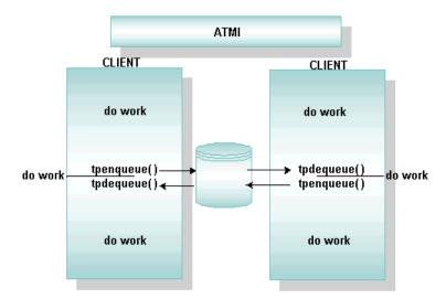
Figure 1-11 Peer-to-Peer Asynchronous Messaging Model
