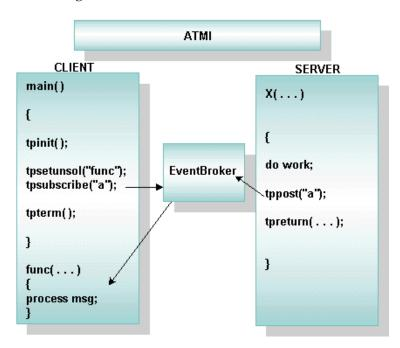
Figure 1-10 Using Event-based Communication
