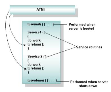
Figure 1-2 Tasks Performed by a Server
