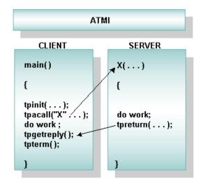
Figure 1-5 Using Asynchronous Calls
