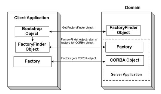
Figure 1-5 How Client Applications Use the FactoryFinder Object
