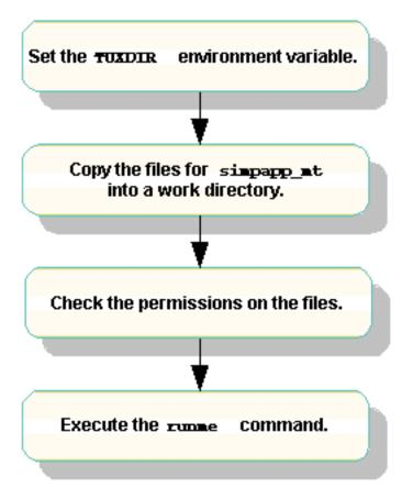
Figure 4-3 Process for Building and Running simpapp\_mt
