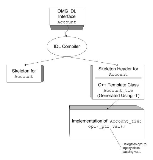
Tie classes are transparent to the client application. To the client application, the tie class appears to be a complete implementation of the object that the client application invokes. The tie class delegates all operations to the legacy class, which you provide. In addition, the tie class contains the following:
