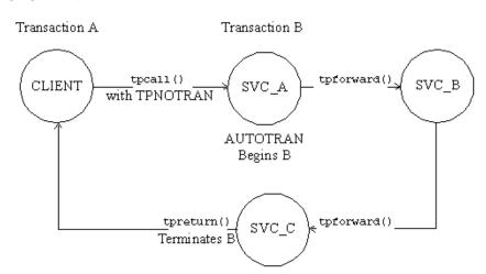
Figure 11-1 Transaction Roles of TPFORWAR and TPRETURN with AUTOTRAN
