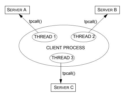
Figure 10-1 Sample Multithreaded Process
