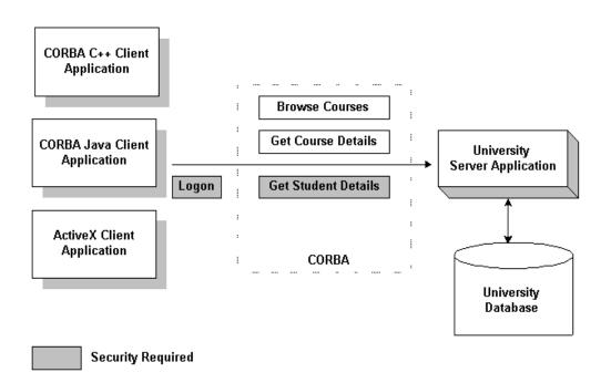
Figure 3-2 How Password Authentication Works
