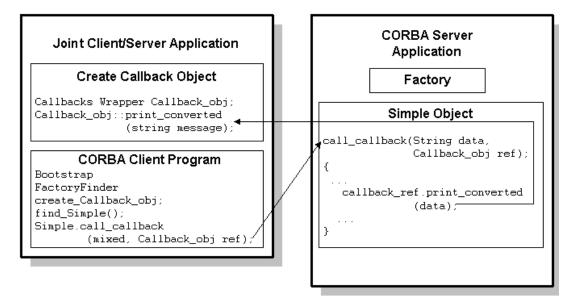
Figure 3-1 The Concept of a Joint Client/Server Application
