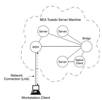
Figure 1-1 BEA Tuxedo ATMI Workstation Component Operation
