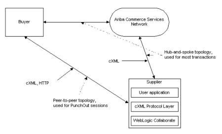
Figure 1-1 WebLogic Collaborate cXML Architecture
