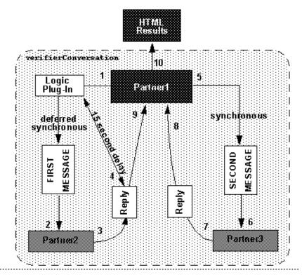
Figure 4-1 Diagram of the Messaging API Sample Conversation
