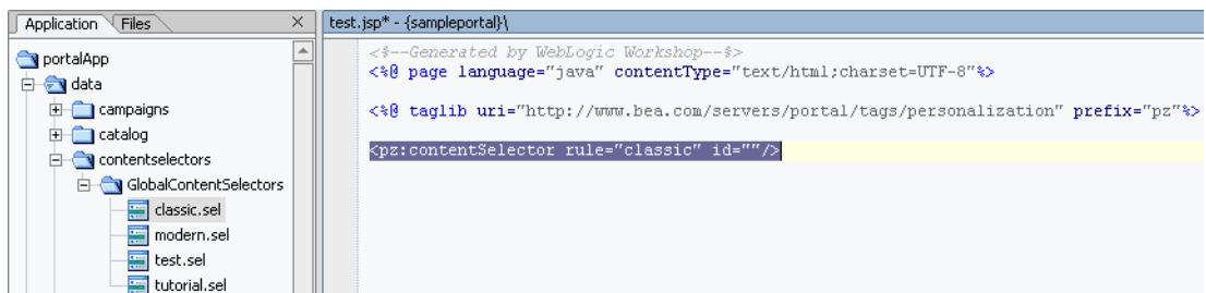
Figure 3-1 The two parts of a content selector: a content selector file and a JSP tag
