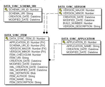
Figure 8-7 Entity-Relation Diagram for WebLogic Portal Data Synchronization
