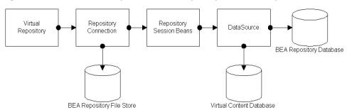
Figure 1-3 Architecture of a Filesystem-based BEA Repository that uses Library Services
