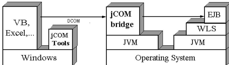
**Figure 2-2 Runtime installation for a typical DCOM late bound implementation.**
