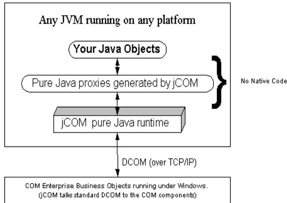
**Figure 1-1 WebLogic jCOM works with any Java Virtual Machine, on any platform, and requires no native code.**
