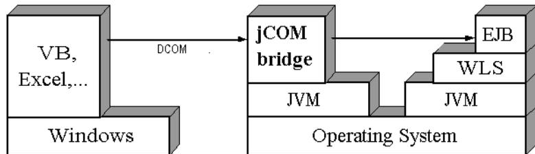
**Figure 2-1 Runtime installation for a typical DCOM zero client implementation.**
