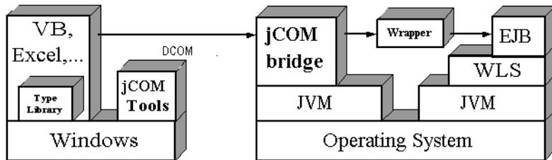
**Figure 2-3 Runtime installation for a typical DCOM early bound implementation.**
