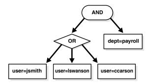
To translate the filter shown in Figure 18–1 into an SQL WHERE clause, you use a recursive function that traverses the tree. The example filter is represented in Oracle Virtual Directory as a hierarchy of Filter objects, which contain collections of other Filter objects to create a traversable tree. The filter shown in Figure 18–1 will have the object model shown in Figure 18-2, where the name of the class used to represent the filter element is below the operation or operand:
