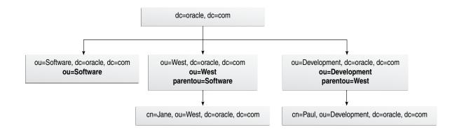
Figure 4–3 shows an example of how the DynamicTree plug-in, with the parentEntryType parameter set to 1 and the attributeName parameter set to parentou, transforms the source directory's flat hierarchy shown in Figure 4–2 into a layered hierarchy in Oracle Virtual Directory.
