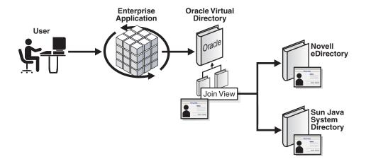
Figure 2–1 Example Simple Join for Authentication
