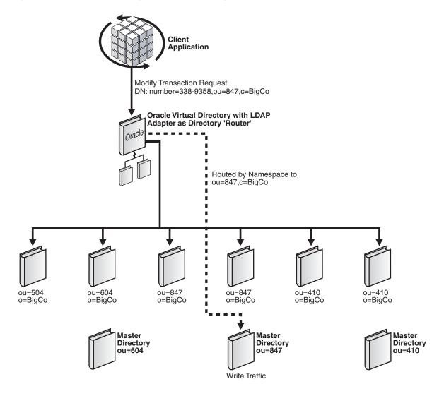
If a flat hierarchy is needed, for example, where all entries appear to be under the same parent, you can choose to either parse the relative distinguished name (RDN), which is the left-most distinguished name or DN component, or to use prefetch operations. If the RDN component can be parsed, then routing could be established through the use of a plug-in that parses the RDN to make routing decisions, as shown in Figure 1–9.
