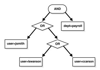
In Figure 18–3, the OR operation is broken up into two separate OR operations. The final WHERE clause from the filter is ((user=jsmith) OR ((user=lswanson) OR (user=ccarson))) AND (dept=payroll). The LDAP prefix notation has been transformed into a SQL like infix notation with only two operands per operation. Example 18–8 shows the source code for the transformation:
