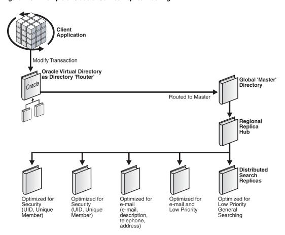
Figure 1–5 Example of Class of Service Replica Indexing
