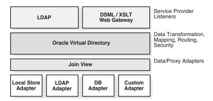
The first layer is Oracle Virtual Directory's listener layer where socket-level protocol is spoken. Oracle Virtual Directory provides two types of listeners: LDAP and HTTP. Both listeners support SSL/TLS on top of their basic protocols. The LDAP layer also provides the ability to support LDAP-SASL to support digital certificate authentication.
