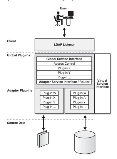
Plug-ins are arranged to form chains. When Oracle Virtual Directory receives a request, the request passes through Oracle Virtual Directory in the following sequence (as shown in Figure 4–1):
