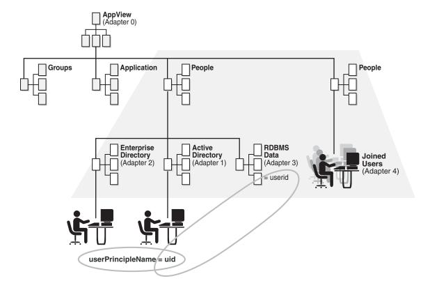
Lastly, because we want to use Adapter 1 for authentication rather than the primary adapter (Adapter 2), you set the bindadapter setting to 1, causing the Join View Adapter to test authentication against the joined adapter rather than the primary adapter.
