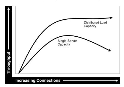
Figure 1–7 Diminishing Throughput Due To Establishing Connections
