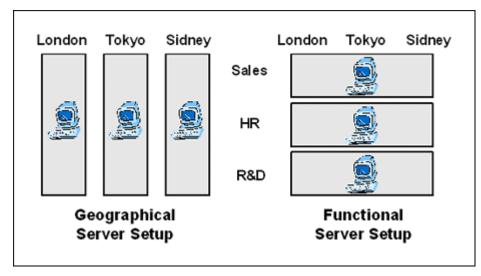
Figure 4-5 Horizontal vs. vertical server setup
