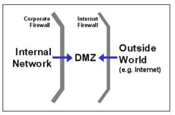
The main purpose of a DMZ is to prohibit any direct data transmission between the Internet and the secure core network. All data must first go through servers in the DMZ, which means there is an extra line of defense against unauthorized access.
