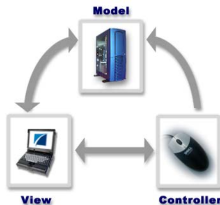
Figure 2 Model/View/Controller (MVC) Architecture
