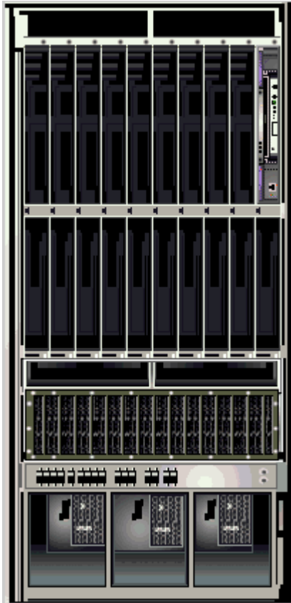
FIGURE 5-10 Sun Fire 15K/12K System Controller Physical View—Front
