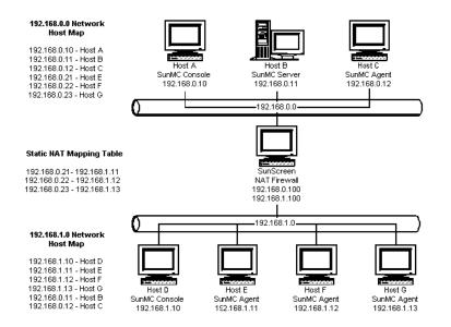
FIGURE D-2 Simple NAT Network Configuration Example
