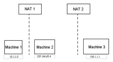
FIGURE D-1 Simple NAT Network Conceptual Diagram
