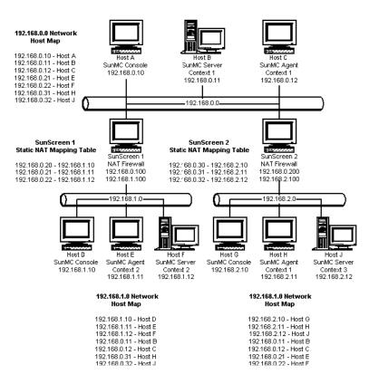
FIGURE D-3 Complex NAT Network Configuration Example
