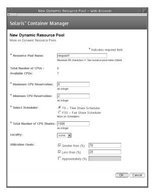
FIGURE 5-1 Resource Pool Window on a Solaris 10 Host
