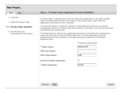
The match expression must be supplied to automatically move the application's processes to the container. This expression is case sensitive. To determine the correct match expression, see "To Determine the Match Expression for an Application" on page 77.
