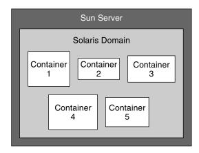
FIGURE 1-2 Example of Containers on a Host
