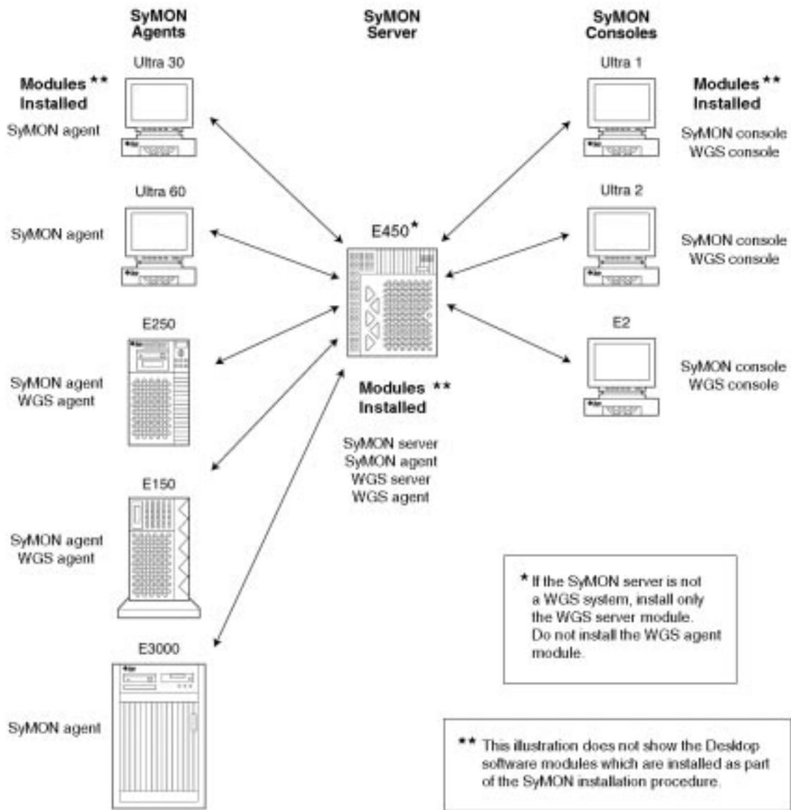
**FIGURE 1** SyMON 2.0 Components Installed on a Heterogeneous Network
